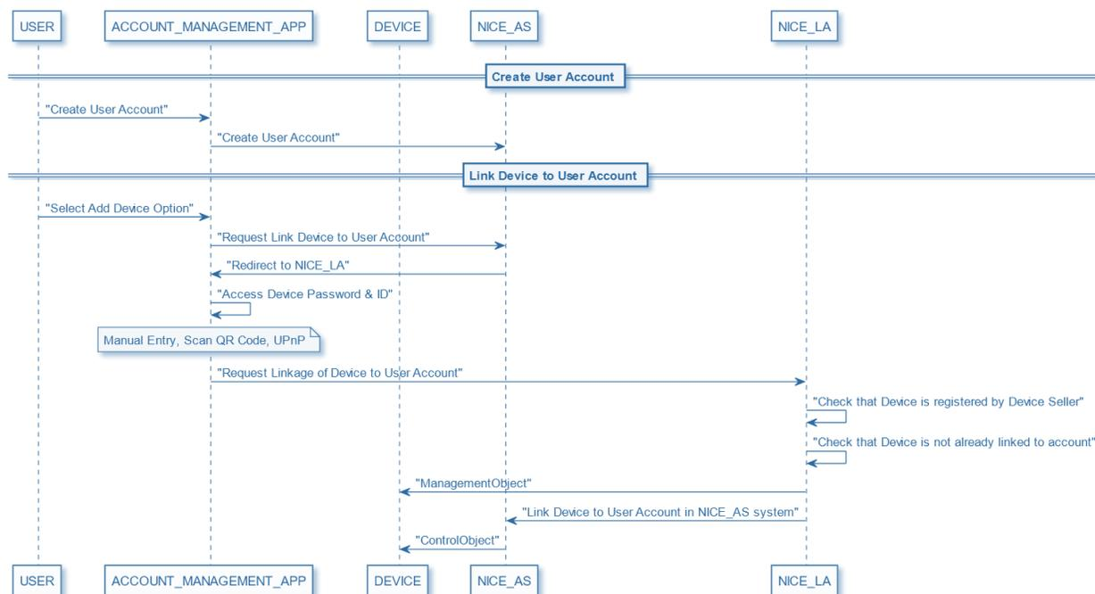
Figure 2. Linking a Device to a User Account
